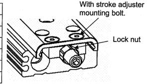
③ Tighten the lock nut according to the tightening torque shown in the table on the right. Insufficient tightening may reduce the positioning accuracy.
