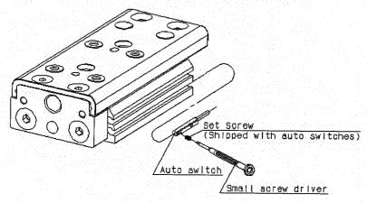
4 Please refer the table below for proper mounting position of the auto switch (when the stroke end is detected).
