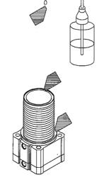
Apply ethanol to clean paper to wipe off dust on O-ring surface.
