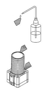
Apply ethanol to clean paper to wipe off dust on O-ring surface and bellows holder surface.
