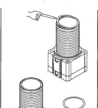
Remove O-ring from the gas release groove with a tool which height is the same as the groove depth. (Mind not to damage O-ring groove)
