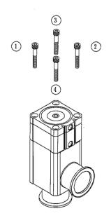
Tighten bolt in numerical order in above drawing. First, hand tighten them evenly until just before O ring is squeezed. Then, tighten them altogether.
