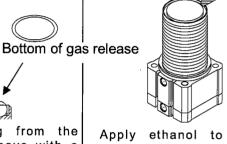
Apply ethanol to clean paper to wipe off the dust in O-ring groove. (Ensure no fiber nor dust are found)
