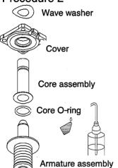
Parts excepting the wave washer and the cover are the service parts. Replace a part which needs to be maintained. Wipe out dust on the surface of each part with a clean cloth (such as BENCOT) soaked into ethanol.
