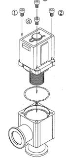
Tighten the bolts in numerical order without a flaw and dust on each part.
