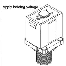
If the coil assembly is applied holding voltage with the above condition (Mount the core assembly on the cover, and fix the coil assembly with the retainer. After that, press the armature assembly until the absorbing position.) when it is assembled again, the armature assembly is fixed at the absorbed position.
