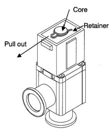
Pull out the retainer to the side with the coil assembly pressed downward.
